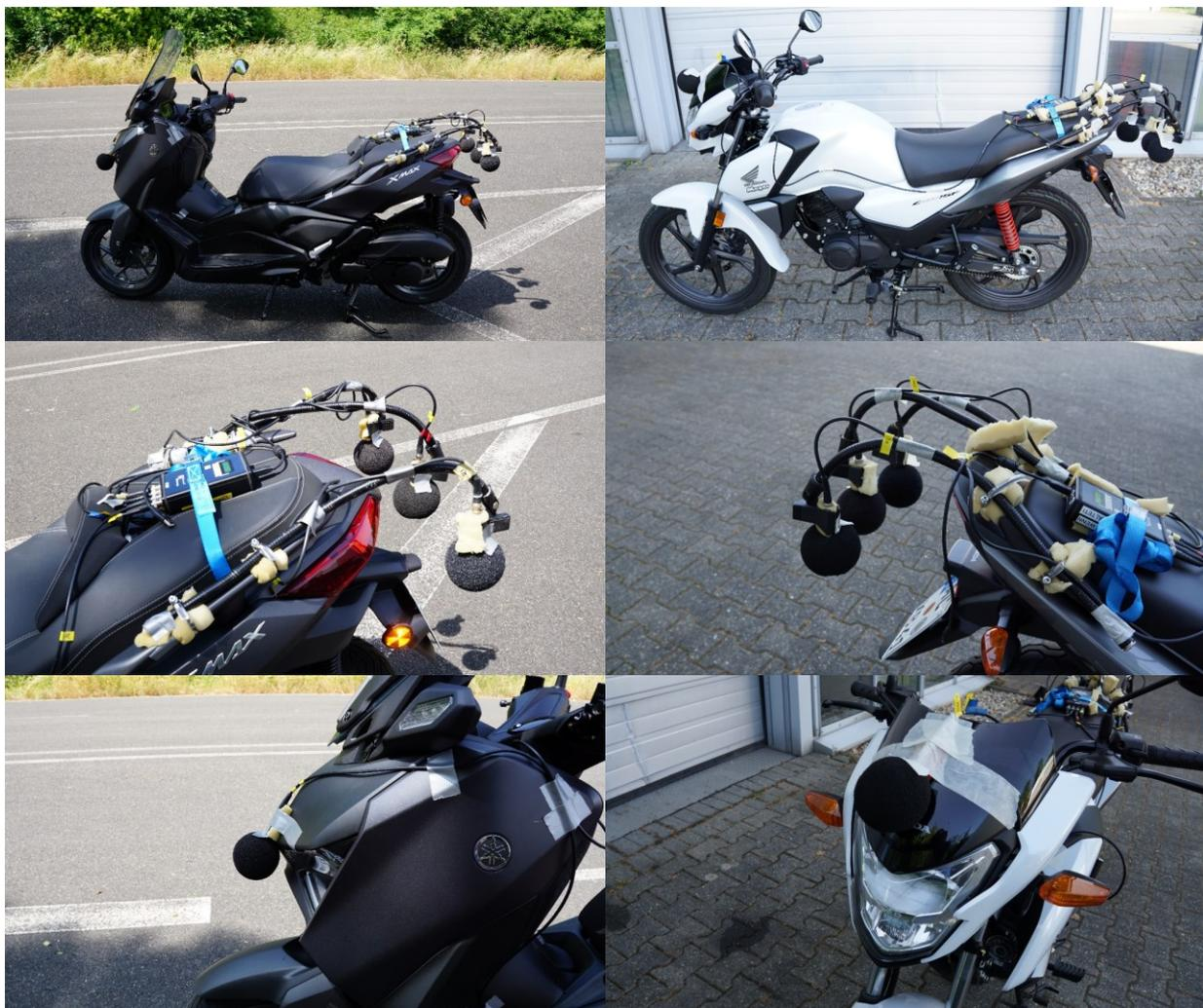
**Figure 4-1:** Microphone setup (three in the back, one in the front) on the vehicles V1 (left) and V2 (right)
